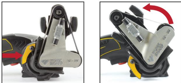
**2** Install Blade Grinding Attachment by aligning the chassis to the keyed "on / off" position then rotate into the "sharpening position".
