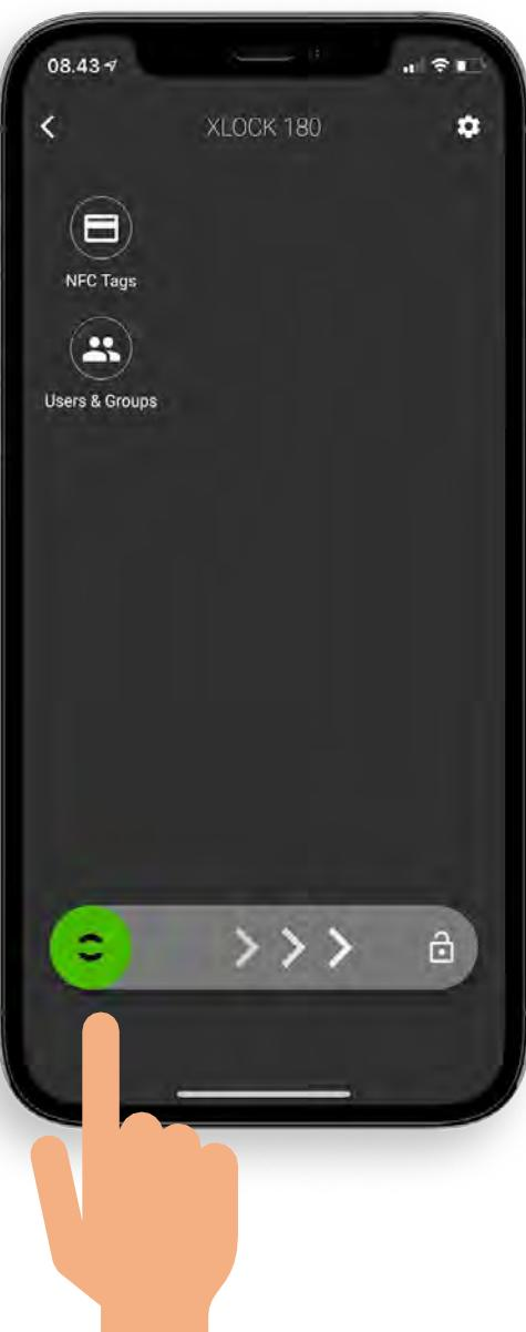
Unlocking with the smartphone and the app is very easy. A swipe to the right unlocks the lock. The reading distance is up to 15 meters. The lock can therefore also be hidden, e.g. installed behind a locker front, invisible. Toggle mode (open/close function) can also be used with the smartphone. This function is activated and deactivated in the lock settings.
