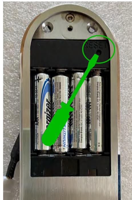
3. Have the XLOCK ready. Press and hold the Reset Button with a screwdriver for 5 seconds. A long sound arises.
