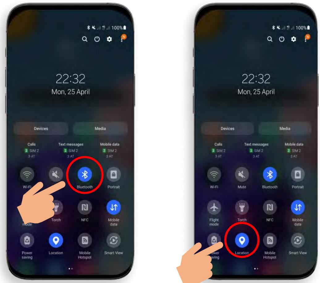
For the programming of an XLOCK lock, the **location** and **Bluetooth** must be activated on your Android device!
