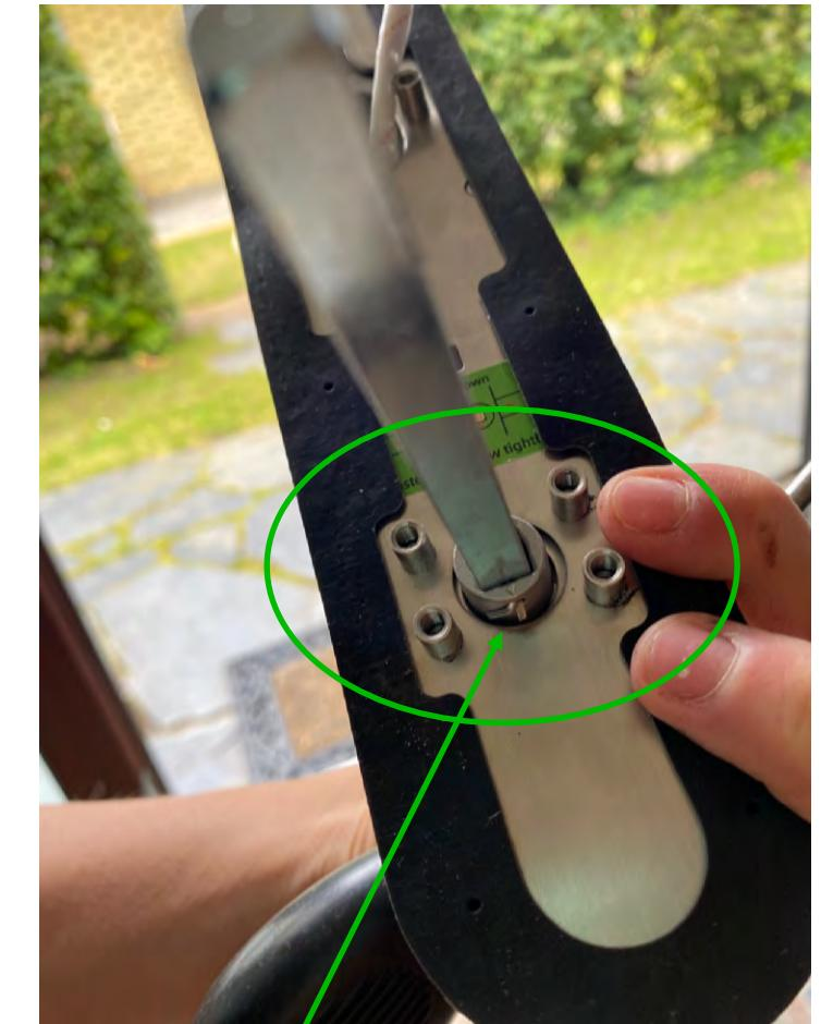
To secure the square shaft it is **very important** to bend the u-clip with the help of a screwdriver.
